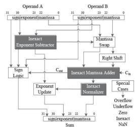
Figure: The inexact single precision floating-point adder architecture.
