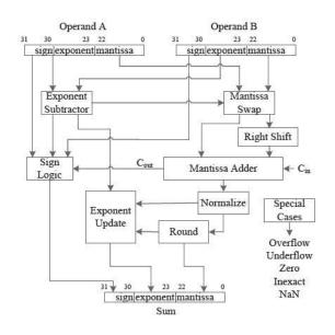
However, as the floating-point adder architecture is substantially different from a fixed-point adder, related logic (addition of an inclusion the normalizer and the rounder) should also be changed.
